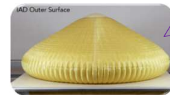
Preliminary Breadboard of the Inflatable Structure
